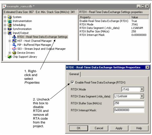
Figure C-3. DSP/BIOS RTDX Control Window in Code Composer Studio v2.20
