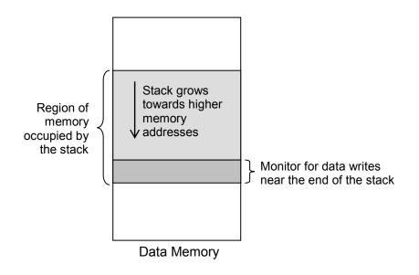
Figure 1. Stack Overflow Monitoring
